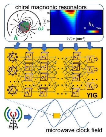
will use nanoscale chiral magnonic resonators [1] as building blocks of artificial neural networks [2]. The power of the networks will be demonstrated by creating magnonic versions of reservoir computers and recurrent neural networks.
