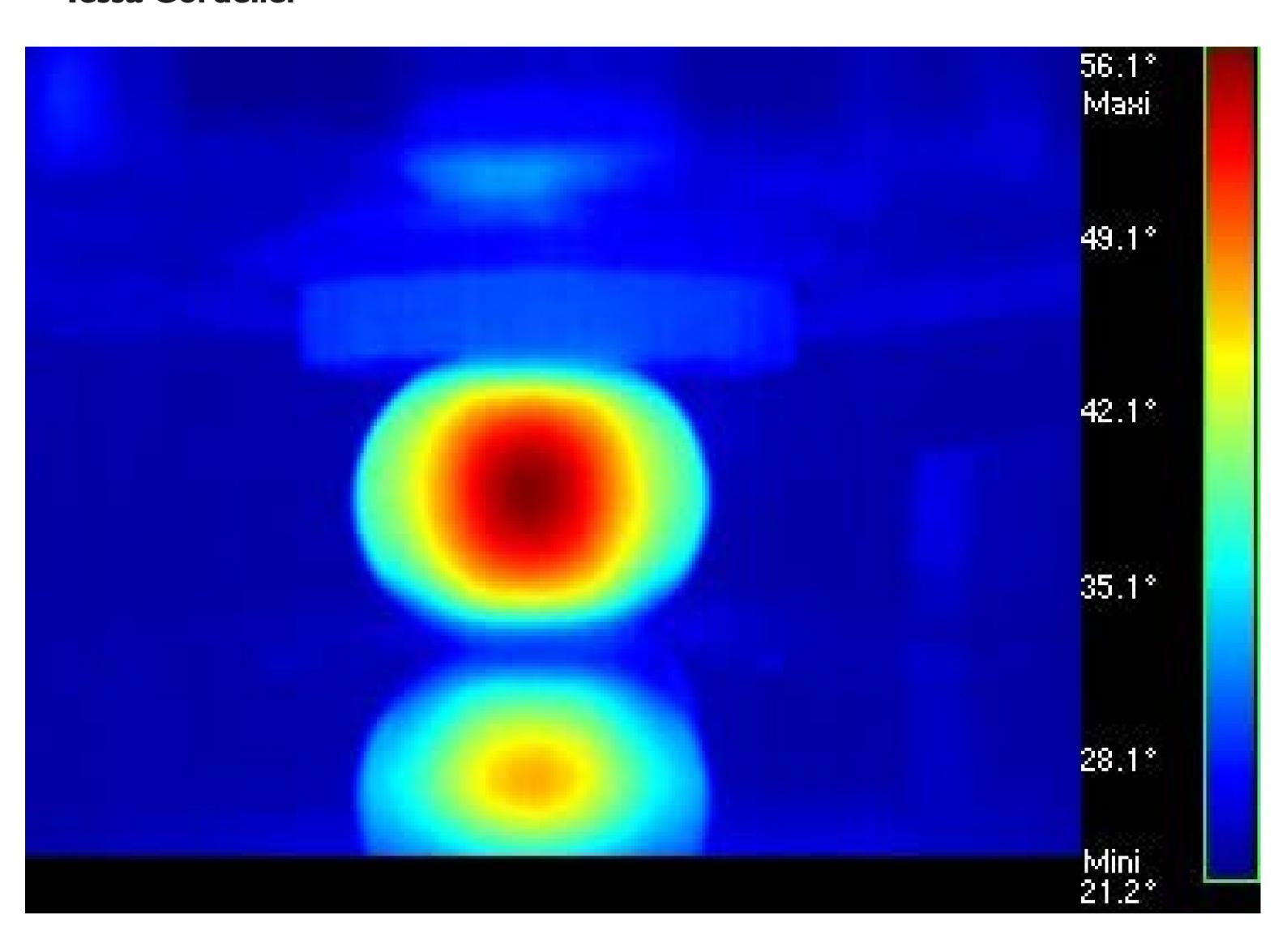
This thermal image shows the temperature increase observed inside a section of polymer cord when subject to repeated compression cycles. This work was conducted to inform the development of the Exeter Tether, a patented mooring tether designed to mitigate peak mooring loads in floating marine renewable energy devices. The polymer under test is EPDM (ethylene propylene diene monomer), and forms a key part of the Exeter Tether core architecture. The long term
