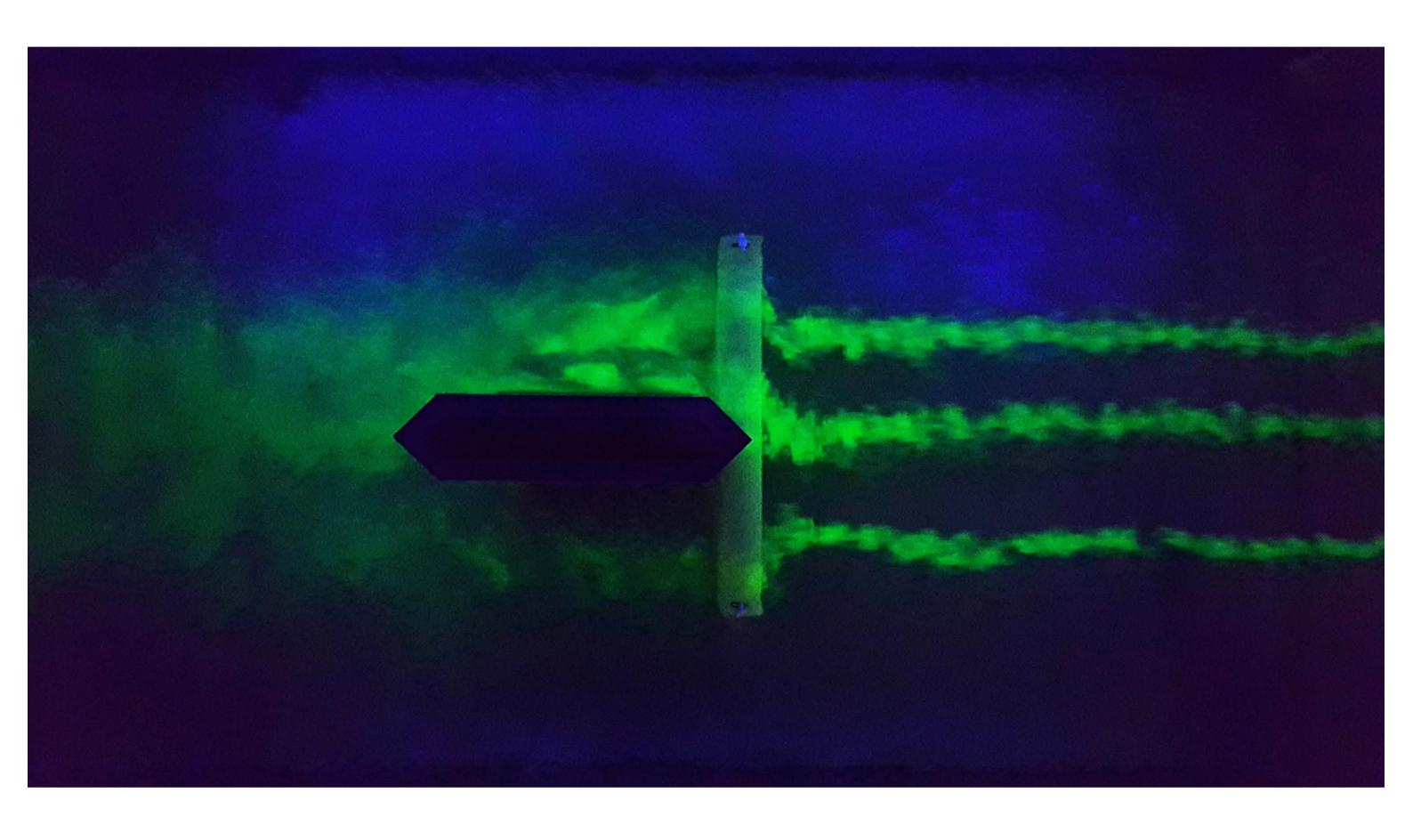
The photo shows plan view of water flow (right to left) visualisation around a bridge pier blocked by a log in a laboratory experiment. This is taken from the preliminary stage of an ongoing project, at Centre for Water Systems, investigating hydrodynamic effects of debris blockage at masonry bridges. Project findings are expected to inform bridge maintenance and enhance resilience of transport infrastructure in the UK.
