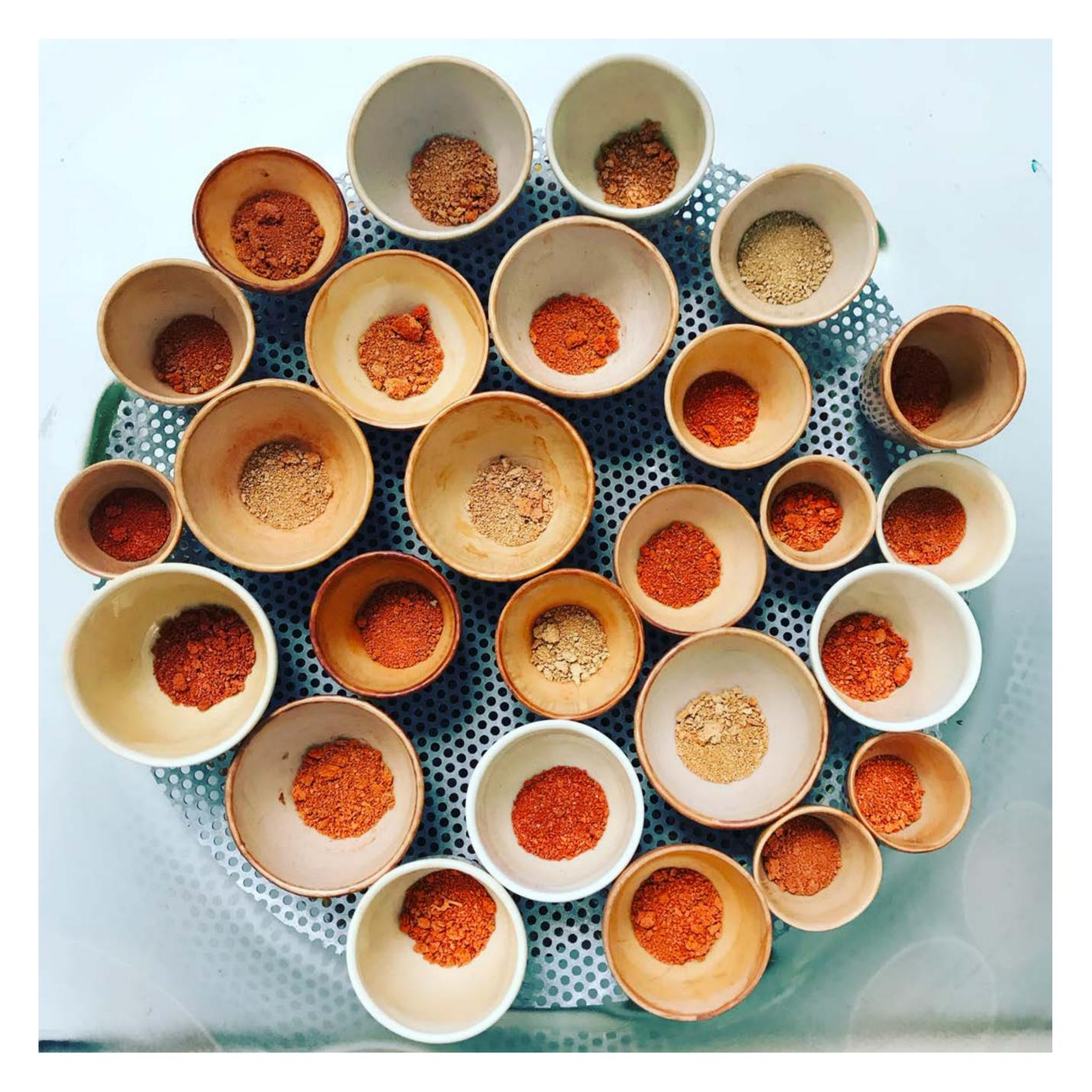
An image of lake sediment samples in crucibles, that have undergone loss on ignition (LOI) analysis. These samples were taken from a lake sediment core that ages 12,000 years. LOI analysis involves burning the sample to temperatures as high as
