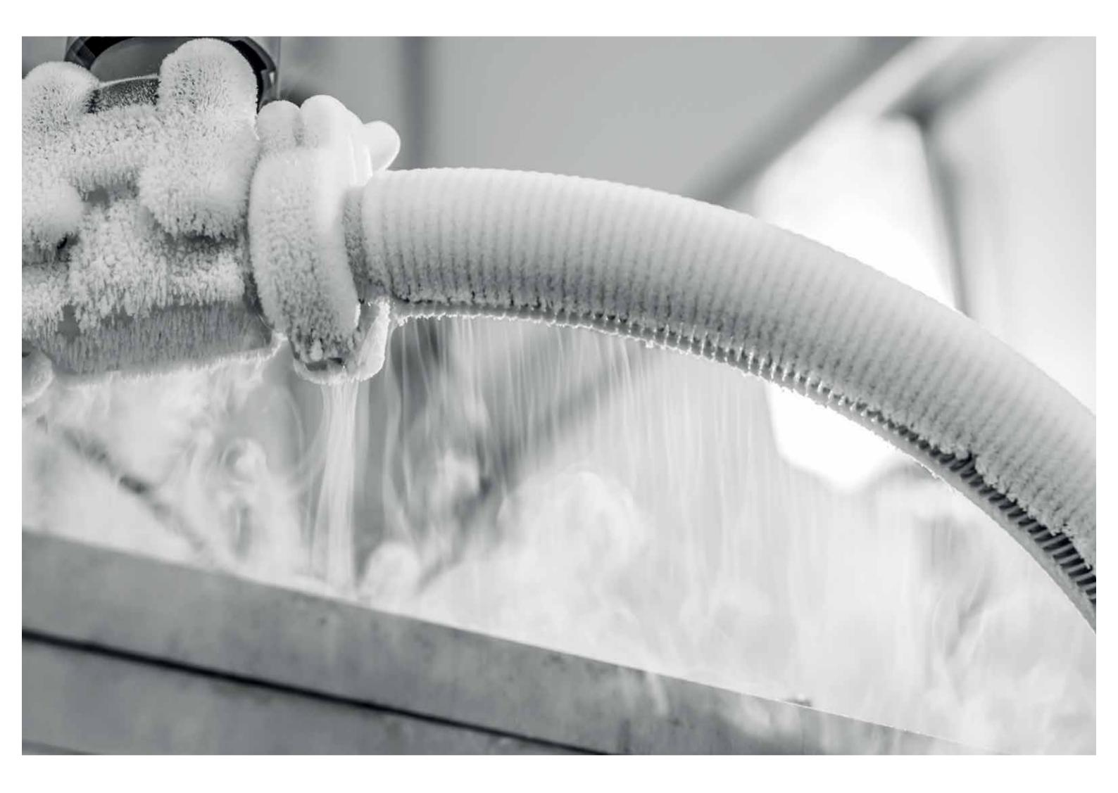
Working at the forefront of technology sometimes means working at the edges of physical observables. In this case, working at temperatures as low as -272 degrees Celsius means approaching the temperature of the coldest parts of the Universe. This can offer beautiful displays such as the one depicted where cold Helium gas flowing through a steel pipe causes the water vapour around it to freeze in beautiful ice crystals. As cold air is denser than ambient
