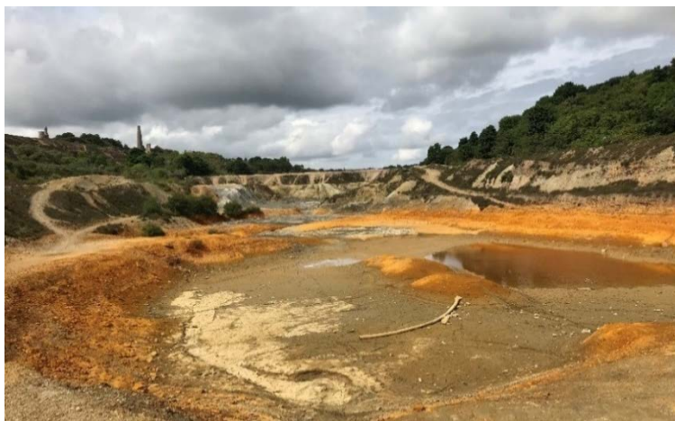
Figure 10 Arsenic-contaminated tin and copper mining waste, Wheal Maid tailings lagoon (Photo courtesy of Karen Hudson-Edwards)
