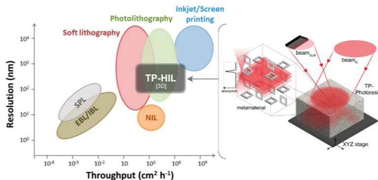
**Fig 1.** Feature resolution versus fabrication throughput showing the location of various lithographic and printing processes, adapted from [2], with added concept of TP-HIL and envisaged performance metrics.
