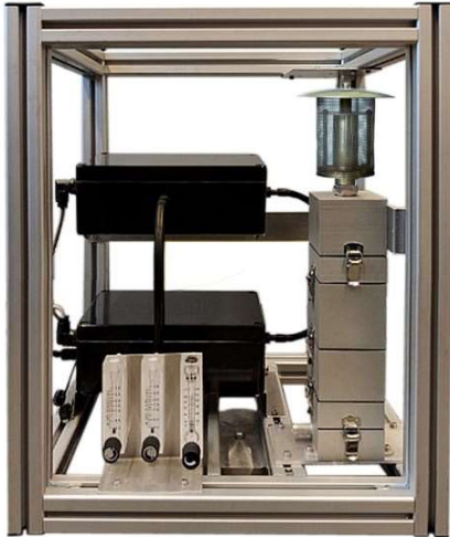
Figure 13 Prototype of new dust-meter DMlex.
