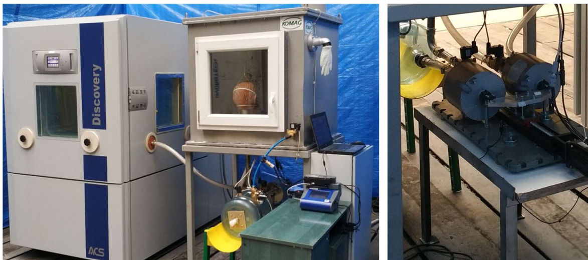
Figure 16 Test stand for assessing the performance of dust masks and filters. Note the test dummy head which is wearing a mask in the experimental chamber. The artificial lungs are shown on the right.
