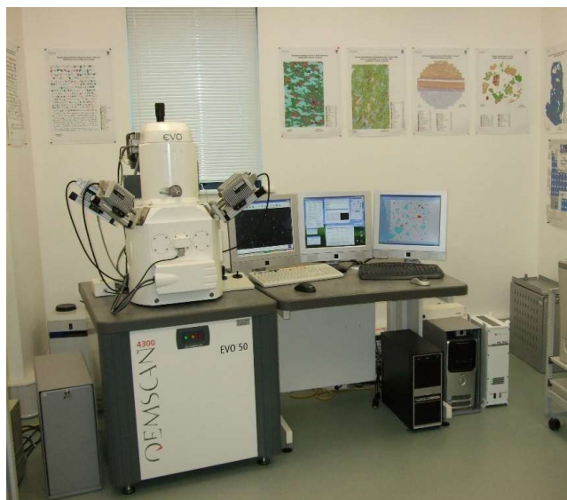
Figure 9 QEMSCAN® automated mineralogical analysis system which can determine the size, shape and mineral associations of up to 100,000 dust particles in 10 hours.
