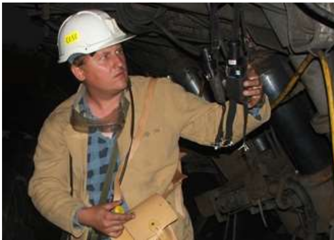
Figure 2 PM 10 sampling underground using a CIP-10 air pump-filter collection system.
