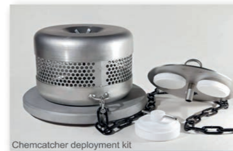
Figure 4 Chemcatcher deployment for pesticide measurement in Cornwall: disks are placed in a cage (above) that is then left in the river and will accumulate contaminants for that duration, thereby giving a picture of the detections in that time period; photo by Tim Ball (SWW).
