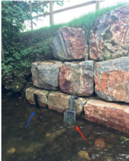
Figure 1 Continuous turbidity sensor (pointed out by the red arrow) and conductivity and pH sensors protected by black tubing (pointed out by the blue arrow) on the River Exe (Pixton gauging station); photo by Paul Henderson.
