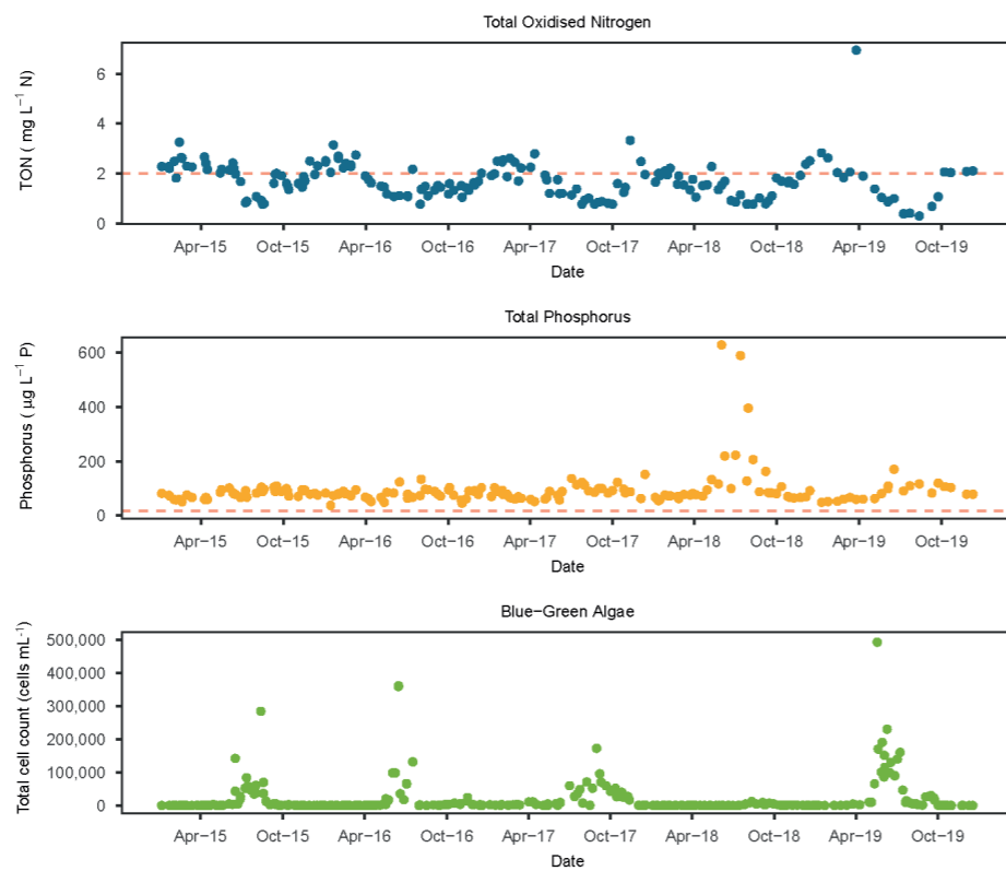
Figure 9 Total Oxidised Nitrogen (top), Total Phosphorus (middle) and blue-green algae cell count (bottom) between 2014 and 2019 in Tamar Lake reservoir; red lines indicate the exceedance limit for each nutrient concentrations.
