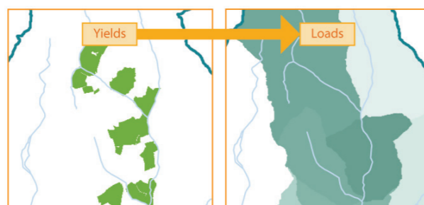
Figure 2 Example of contaminant yields (left) at the farm scale identified by the green areas, leading to calculations of corresponding changes in contaminant loads (right) for the same reach. The darker colours represent greater decrease in loadings.
