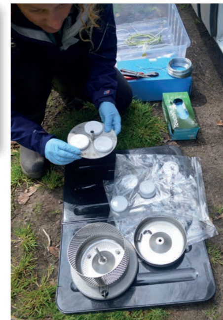
Figure 4 Chemcatcher deployment for pesticide measurement in Cornwall: disks are placed in a cage (above) that is then left in the river and will accumulate contaminants for that duration, thereby giving a picture of the detections in that time period; photo by Tim Ball (SWW).
