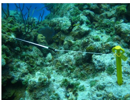
Fig 2.1 | Survey tape attached to marker stake showing 50 cm long 'leader' cord from clip to main tape.
