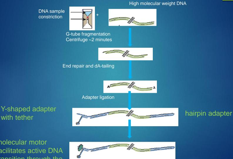
molecular motor facilitates active DNA transition through the nanopore
