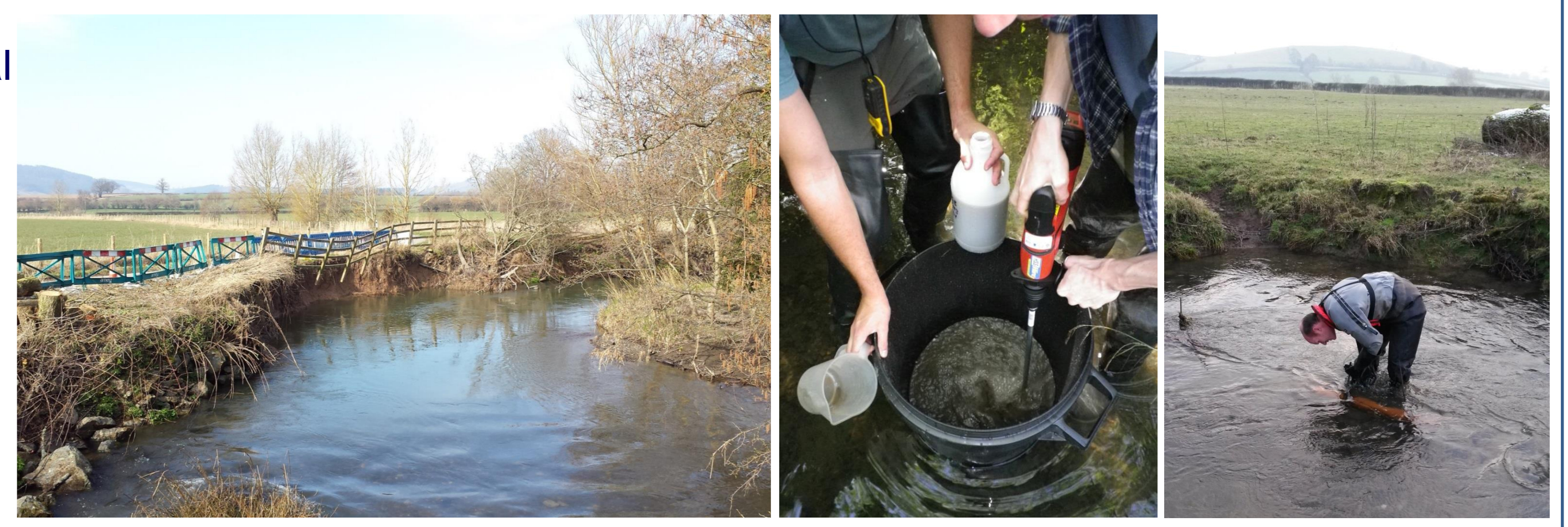
Figure 3 (right): Sampling bed sediment (left), in-situ Phillips suspended sediment samplers (middle) and channel bank erosion (right)
